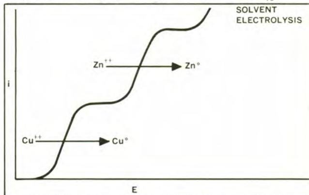
Figure 13. Current-Voltage Curves for a Multicomponent System.
