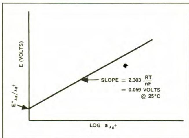
Figure 4. Plot of Potential Versus  $\log a_{Ag^+}$ .
