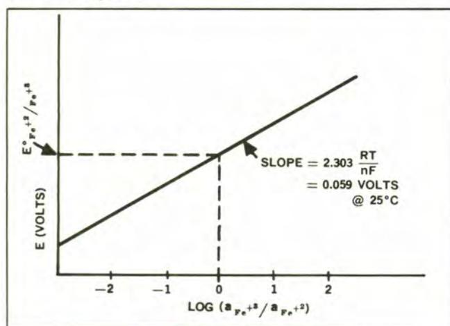
Figure 6. Plot of Potential Versus  $\log a_{Fe^{+3}}/a_{Fe^{+2}}$ .
