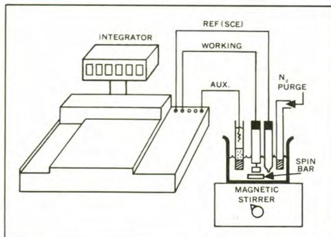
Figure 29. Instrumental Configuration for Controlled Potential Coulometry.
