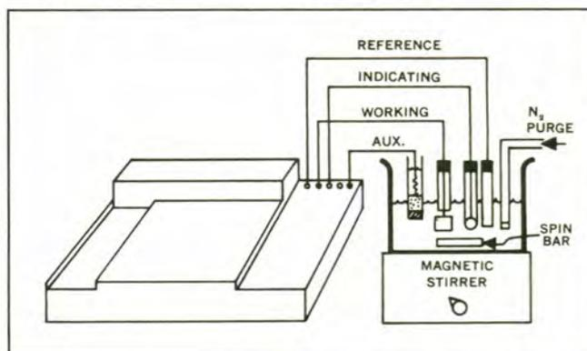
Figure 34. Instrumental Configuration for Controlled Current Coulometry.
