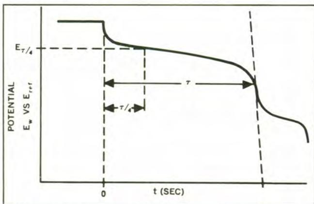
Figure 32. Typical Chronopotentiogram of the Reduction of  $\text{Fe}^{+3}$ .
