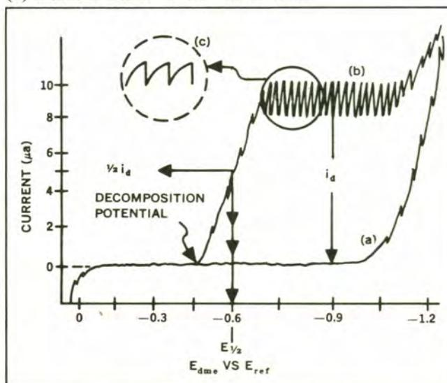
Figure 17. Polarogram of  $\text{Cd}^{2+}$  in 1F HCl.
