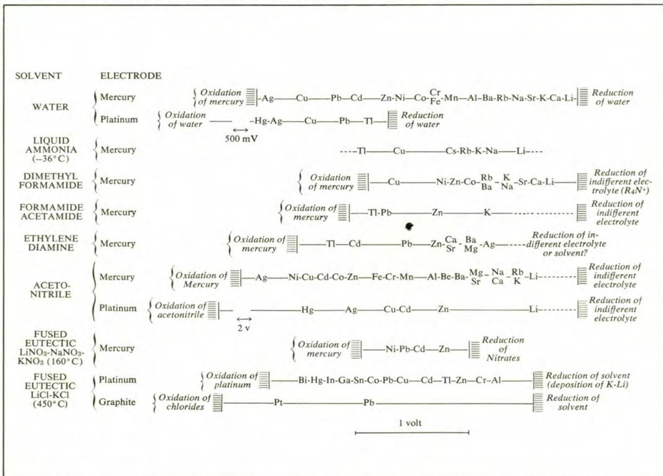
Figure 14. Ranges for Solvent-Electrode Combinations.<sup>1</sup>
