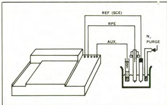
Figure 19. Instrumental Configuration for Solid Electrode Voltammetry.
