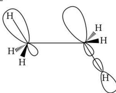
$C - H \sigma^*$  anti-bonding orbital on the other carbon atom is partly responsible. This interaction is greatest when the two orbitals are exactly parallel.
