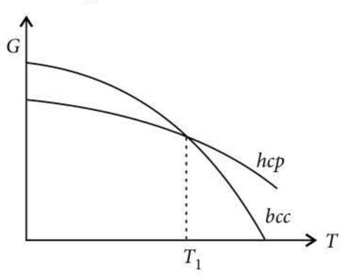
Around 30 metals, show temperature dependent polymorphism. Iron is a unique element. It has a *bcc* modification (alpha iron) in lower temperature range, below 912 °C. Then it changes to *ccp* (gamma iron) and then finally *bcc* (delta iron) again at high temperature before it melts to liquid. The low temperature *bcc* in case of iron is because of reasons, which are beyond the scope of this discussion.
